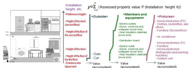
Figure 1 An image of vertical distribution of properties of a building model (detached house)
