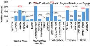
Figure 1: Basic trend of the onset of vehicles becoming stuck
