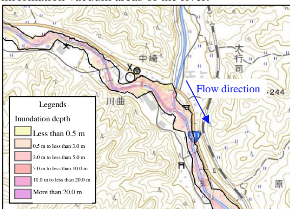
Fig. 2 Simple estimated inundation map (estimated maximum scale: Trial version)
