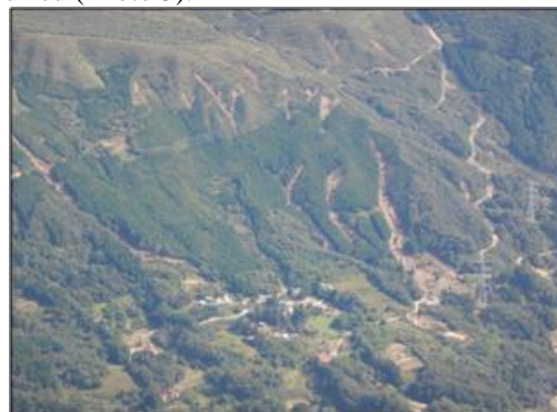
Photo 5 Frequent slope collapse and debris flow (Igu-gun, Miyagi) Mawarigura Area, Marumori-machi, Oct. 17)
