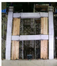
Partial structure test using RC framework + CLT wing walls
