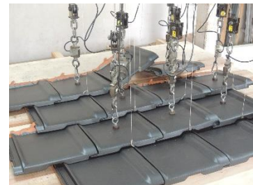
Figure 2: Example of load test on a tile roof (F-shaped tile)
