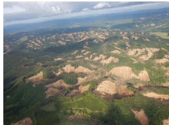
Photo-2 Condition of slope collapse caused by 2018 Hokkaido Eastern Iburi Earthquake
