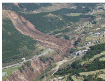
Slope failures caused by 2016 Kumamoto Earthquakes
