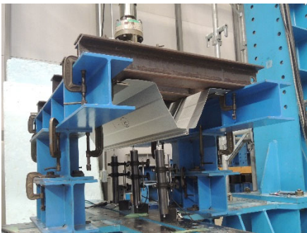
Photo-2. An example of conducting a tensile load test on the joining part of bent board thatching.
