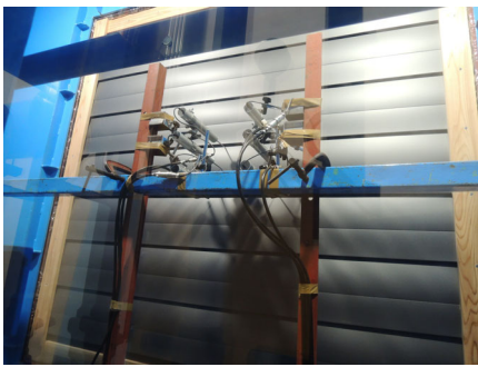
Photo-1. An example of conducting a wind-proof pressure performance test on metal board thatching
