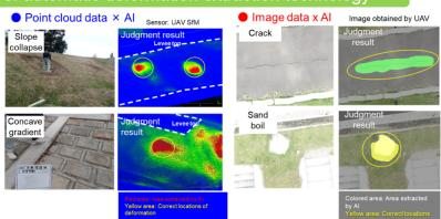
Example of field demonstration of automatic deformation extraction
