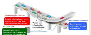
Provide the position, speed, etc. of main lane vehicles to merging vehicles and support merging into main lane safely and smoothly
