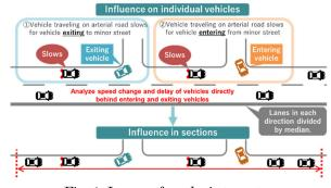
Fig. 1. Image of analysis target
