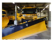
Photo 1: Example of airport snow removal vehicle (snowplow)
