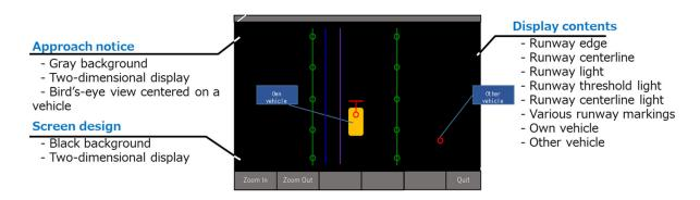
Photo 2: Driver assistance guidance system (on-vehicle monitor)
