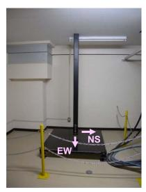
Photo 9.2-3 Scratch board installed on the SI floor
