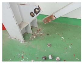
Photo 6.4-4 Fracture of bolts
