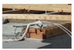
Photo.7.4-5. Failed hold down fastener.
