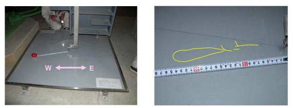
Photo 9.2-23 Trace of displacement of the SI floor on the scratch board
