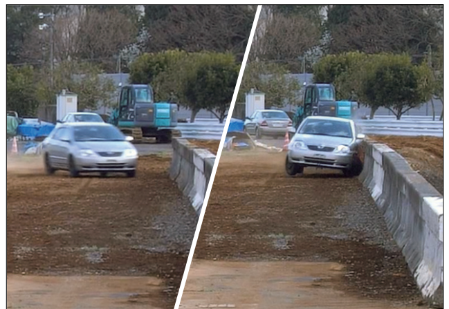
Photo: Testing collision between actual car and protective fence A driver-less car is accelerated by special driving equipment, made to collide with the protective fence at a set collision speed and angle, and the performance of the protective fence is evaluated.
