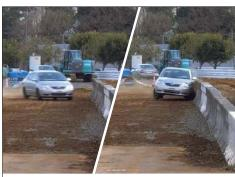
Photo: Testing collision between actual car and protective fence A driver-less car is accelerated by special driving equipment, made to collide with the protective fence at a set collision speed and angle, and the performance of the protective fence is evaluated.
