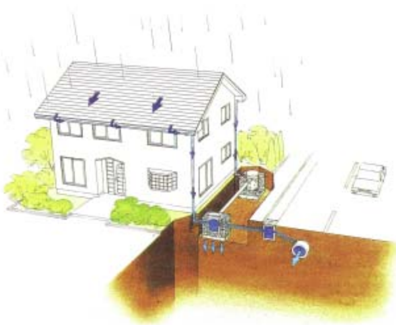
Infiltration inlet installed in front of a house
