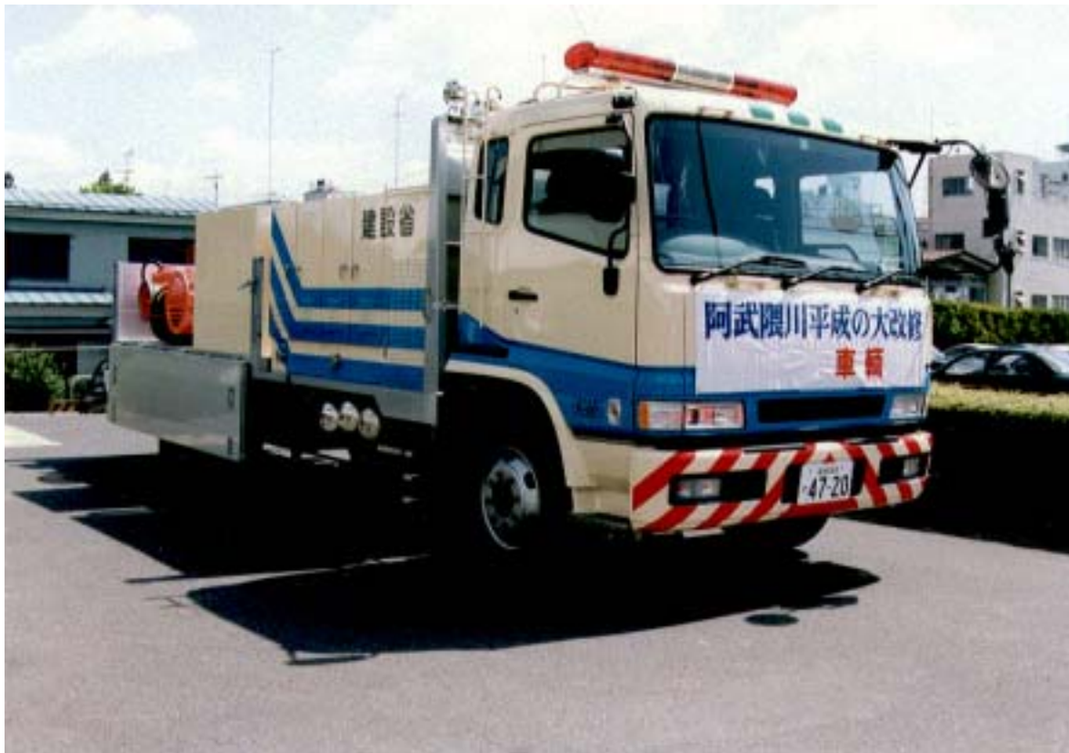
Drainage pump vehicle deployed in Sukagawa City
