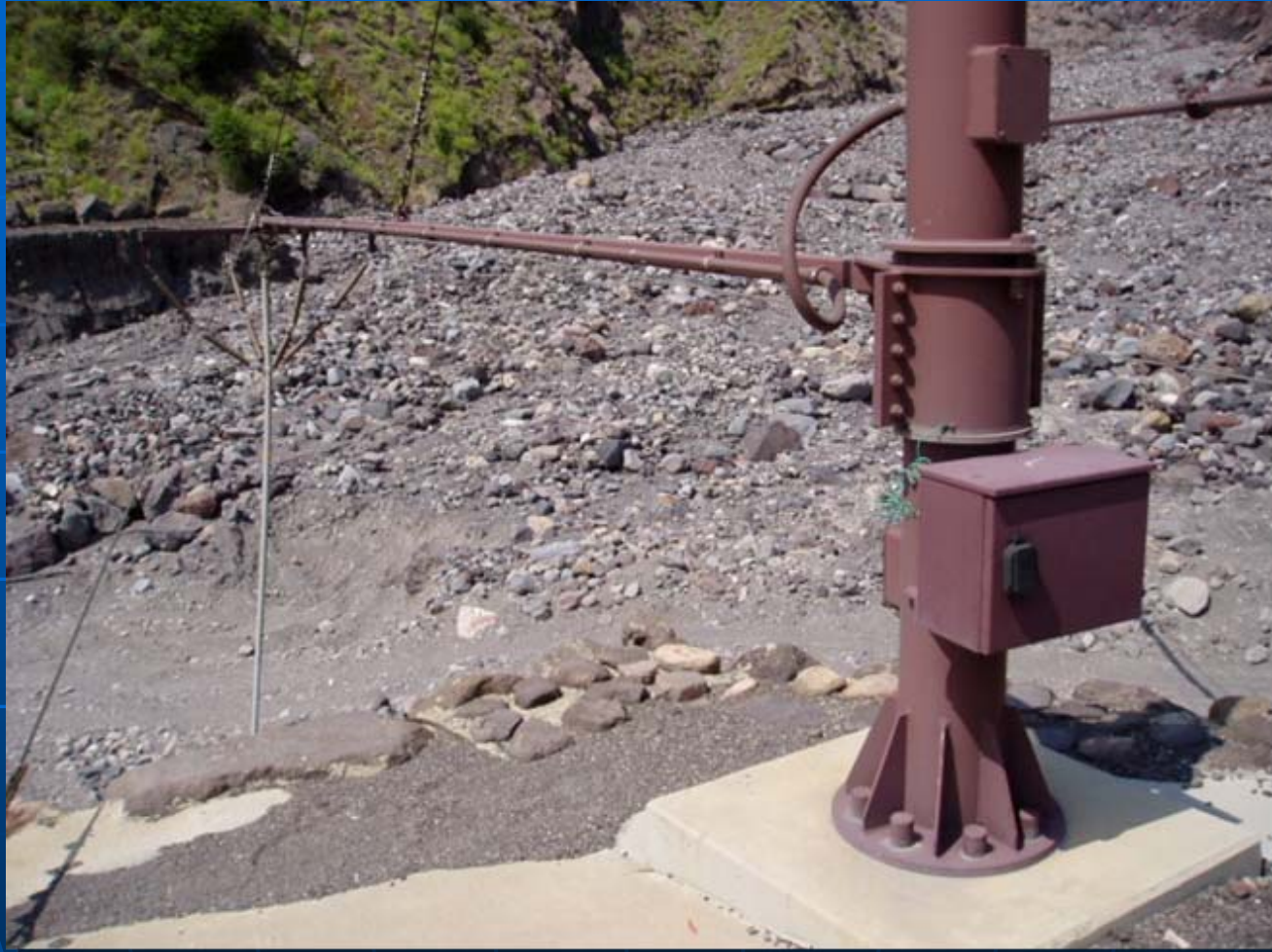
Touch sensor (Swinging rod-type surface detecting sensor)
