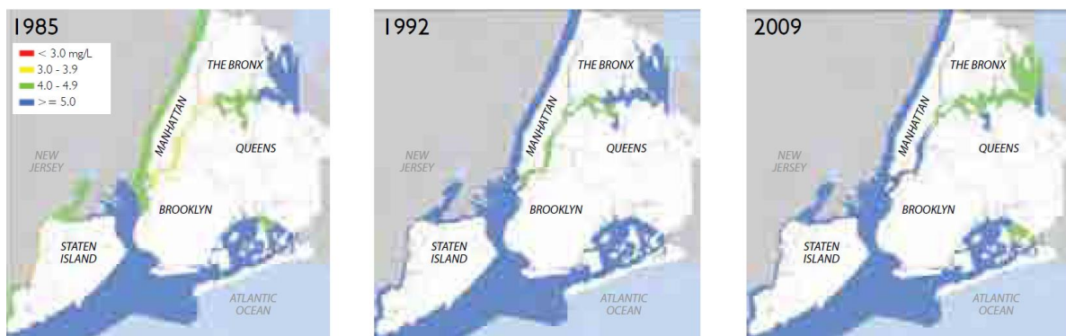
Figure 1: Harborwide Water-Quality Improvements from 1985 to 2009: Summer average for dissolved oxygen in bottom waters, showing increasing oxygen levels.
