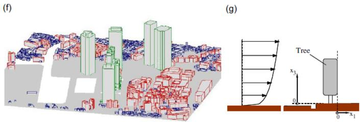
Fig. 1. Seven test cases for cross-comparison. (a) Test case A (2:1:1 square prism); (b) Test case B (4:4:1 square prism); (c) Test case C (Simple city blocks); (d) Test case D (High-rise building in city); (e) Test case E (Building complexes with simple building shapes in actual urban area); (f) Test case F (Building complexes with complicated building shapes in actual urban area); (g) Test case G (Two-dimensional pine tree).
