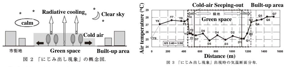
Fig. 2 Schematic image of seeping-out phenomena. Fig. 3 Temperature distribution along cross-section line when seeping-out phenomena appeared.
