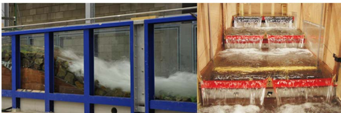
Figure 49 2D Physical model research soil protection (source: Deltares)
