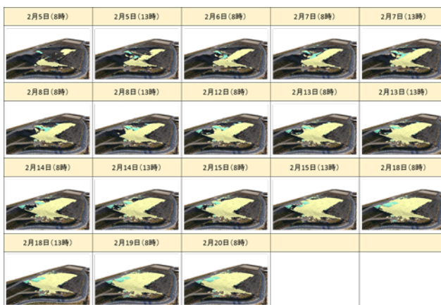
Figure 11. Continuous display of earthwork amount for each day in Site-A
