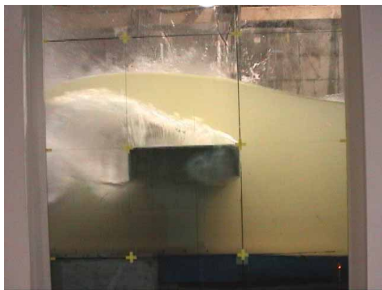
Photo 1 Solitary wave striking the bridge girder model ( H_0=40 [cm], h=17.5 [cm]).
